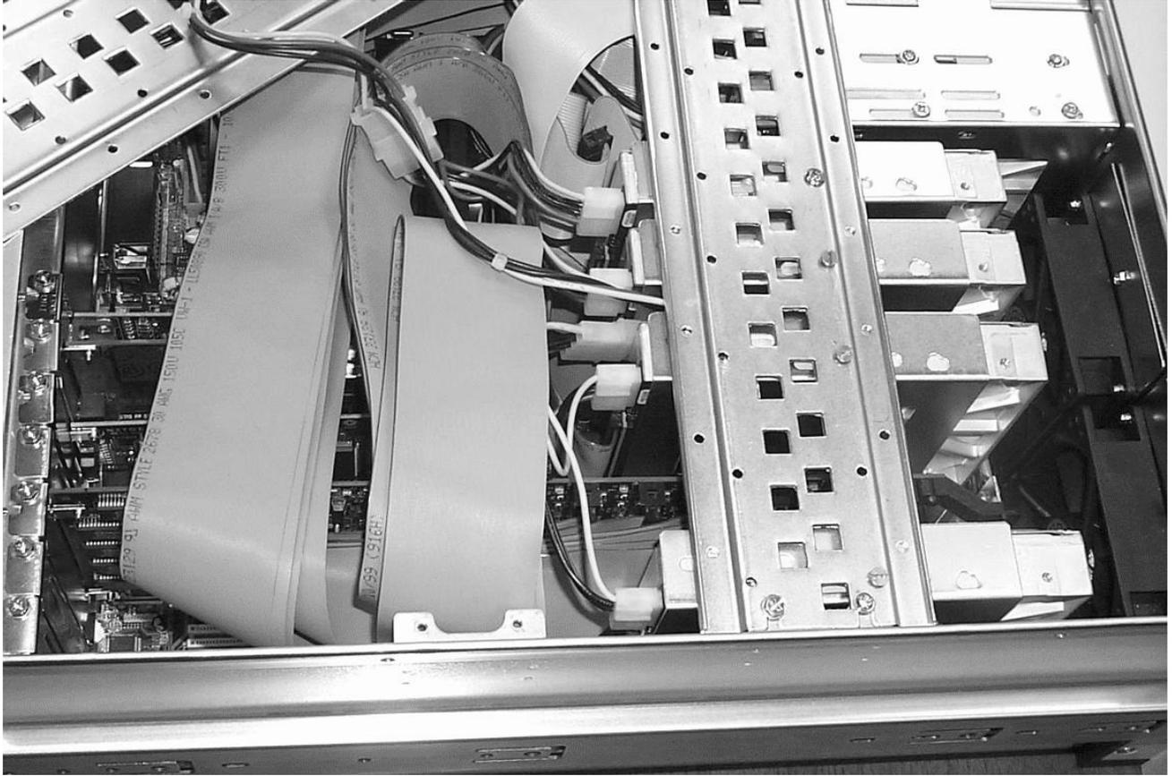
Figure 2: Top/side view of the system. Four 40GB EIDE disk can be seen on the right with the 3ware card between the bottom two. One of the CPUs can be seen on the top left above the four cards (1 AGP graphics card, 1 100Mb NIC, 1 1000Mb NIC, and the 3ware card).
