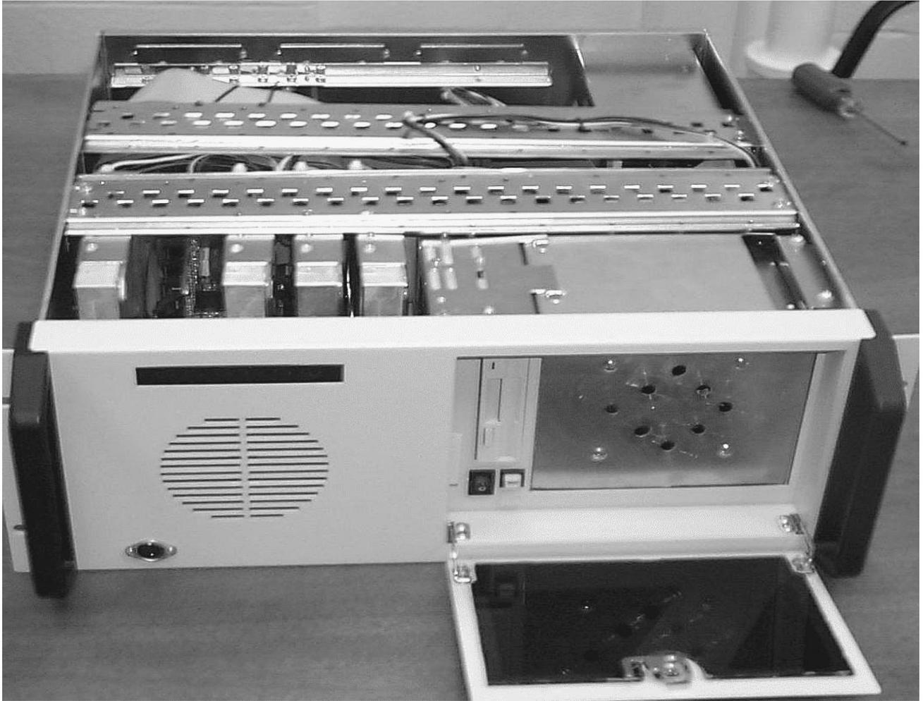
Figure 1: Top/front view of system. Four 40GB EIDE disk can be seen on the left with the 3ware card between the last two on the left. Four others are stacked horizontally behind the homemade fan/copper plate arrangement. The 13GB system disk is next to the floppy drive.
