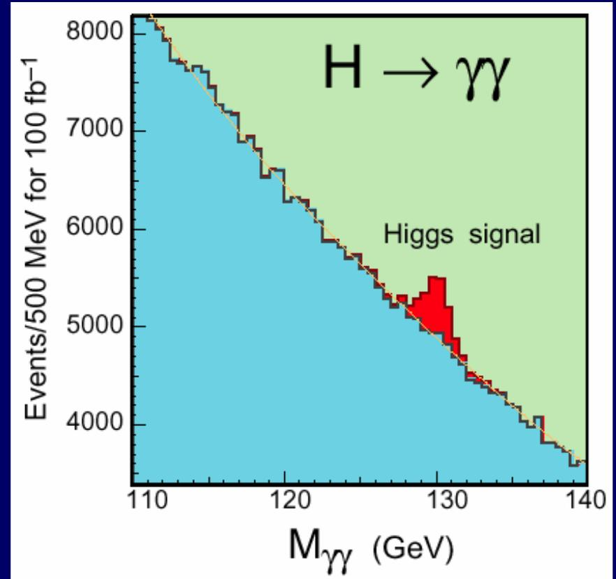
Excellent calorimeter provides 1 GeV mass resolution which allows a peak to be seen
