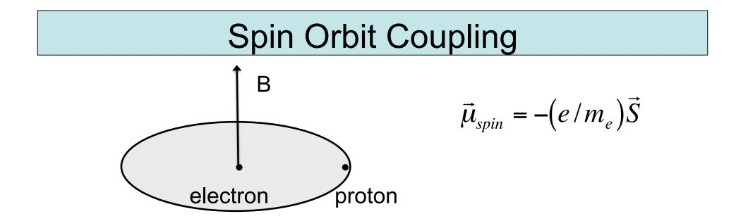
In electron's rest frame, proton circulates around it and the electron sees a magnetic field; the magnetic field is proportional to **L**, the orbital magnetic field.  $B \propto L$
