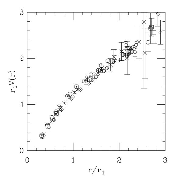
Dimensionless combination  $r_1V(r)$  vs  $r/r_1$  from data sets matched at  $(m_{PS}/m_V)^2 = 0.48$ . Symbols are crosses for  $N_c = 2$ , octagons for  $N_c = 3$ , squares for  $N_c = 4$  and diamonds for  $N_c = 5$ .
