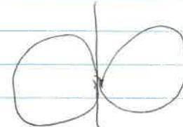
$$R \text{ in ohms} = 30 c \cdot R_{cgs} = 5(kd)^2 \Omega$$
