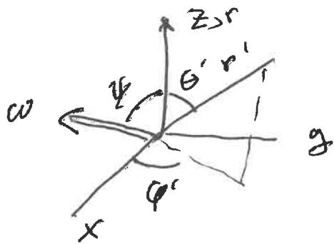
$$\text{so } \vec{\omega} \times \vec{r}' = \omega \begin{vmatrix} \hat{x} & \hat{y} & \hat{z} \\ \sin \psi & 0 & \cos \psi \\ \sin \theta' \cos \varphi' & \sin \theta' \sin \varphi' & \cos \theta' \end{vmatrix}$$
