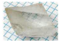
A calcite crystal laid upon a graph paper with blue lines showing the double refraction
