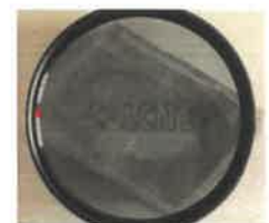
Doubly refracted image as seen through a calcite crystal, seen through a rotating polarizing filter illustrating the opposite polarization states of the two images.
